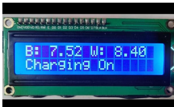
Fig. 5: Voltage observed at receiver side
