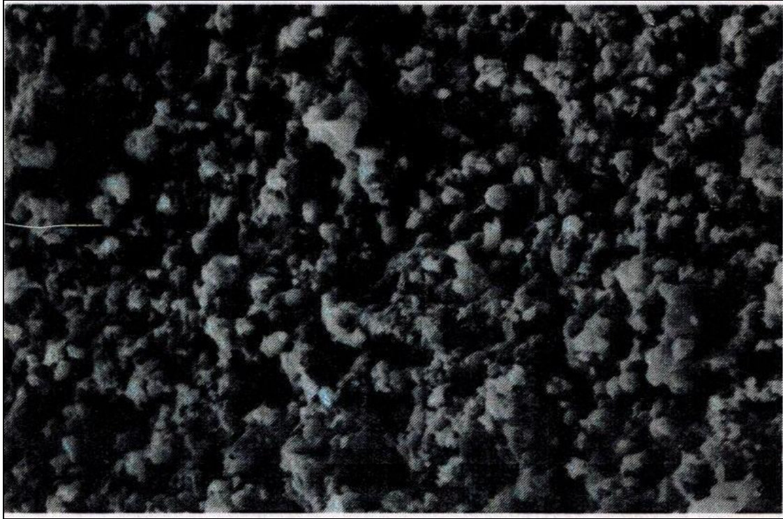
Figure 4: SEM Micrograph Of nHAp from Crayfish Mandible (CFHAp)
